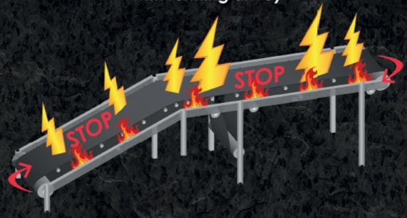
Category 3 – conveyor belts for general applications with no risk to propagation of fire in case of spontaneous ignition due to friction against support structures or driving drums.
