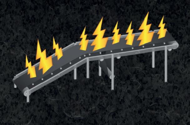
Category 1 – conveyor belts for general applications with no risk to ignition of conveyed materials or adjacent areas due to electrostatic sparking. No protection against inflammation of belts.
